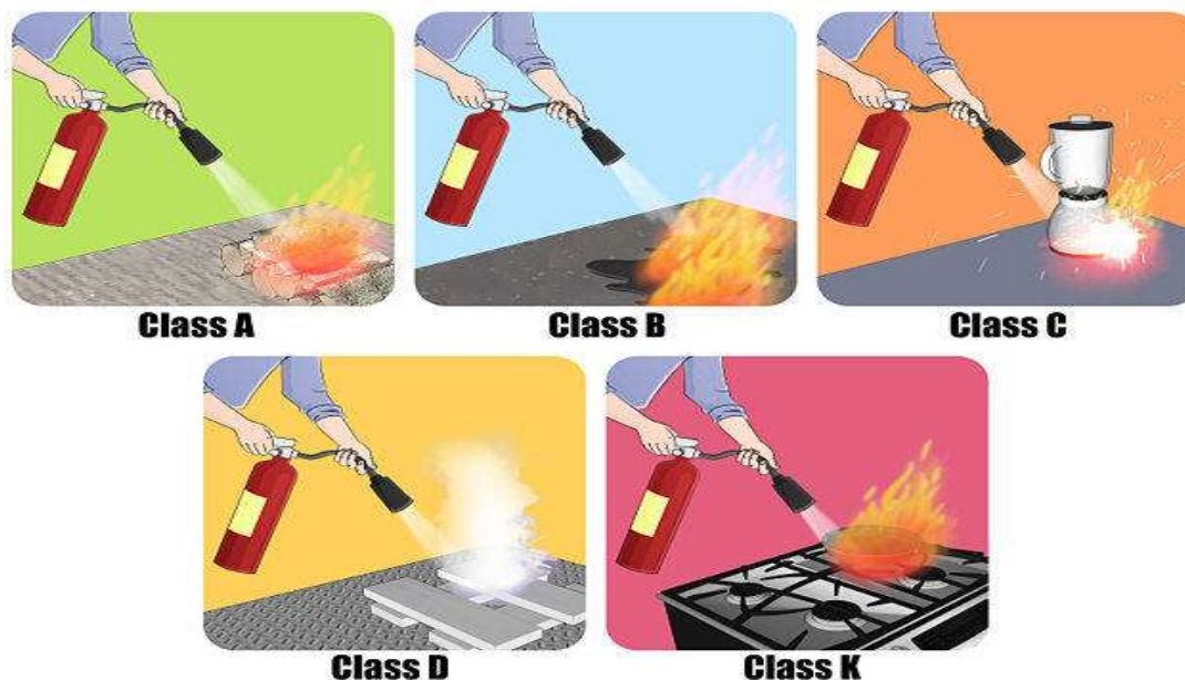
Figure 7.2.2 Classification of Fire Extinguisher
